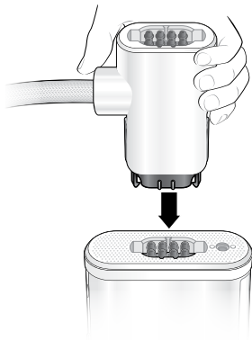
Figure 3.2.b. Connecting the Bilateral Adapter to the Controller Unit
